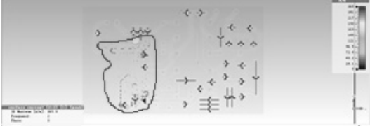
Fig. 7. The surface current distribution diagram of PCB(Port1 2GHzb).
