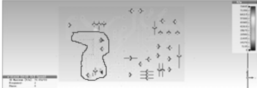
Fig. 6. The electric field distribution diagram of PCB(Port1 2GHzb).
