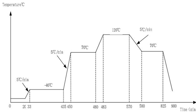
Figure 3. Temperature profile of the device
