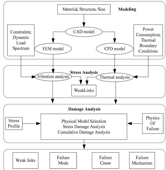
Figure2. Electronic product failure mechanism analysis method process
