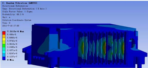
Figure 8. Root mean square value of displacement cloud picture of the device at takeoff state
