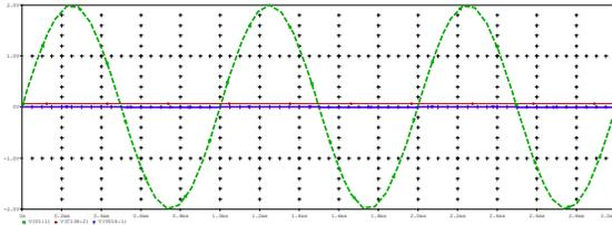
Figure 12. Simulation result of short fault effect analysis of C125
