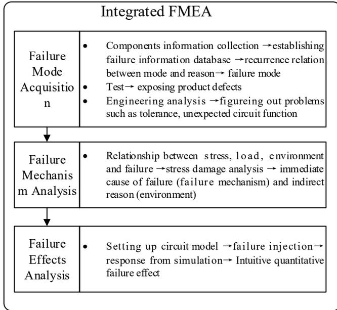
Figure 1. Implementation process of integrated FMEA method
