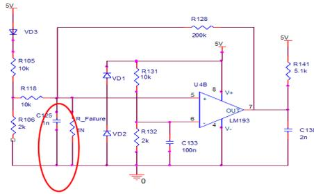
Figure 11. Simulation circuit schematic diagram of short fault effect analysis of C125
