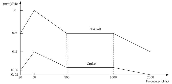
Figure 4. Vibration profile of the device
