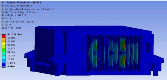
Figure 7. Root mean square value of acceleration cloud picture of the device at takeoff state
