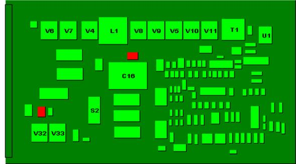
Figure 9. Failure point in the front of the AC-DC's PCB
