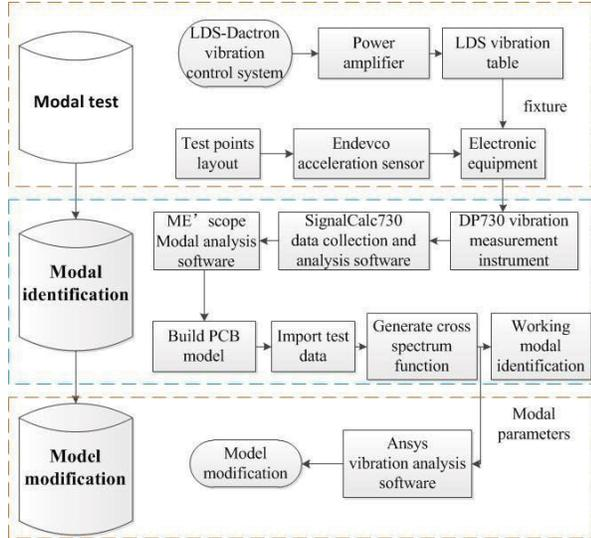
Fig. 1. The vibrostand-driven working modal test system.
