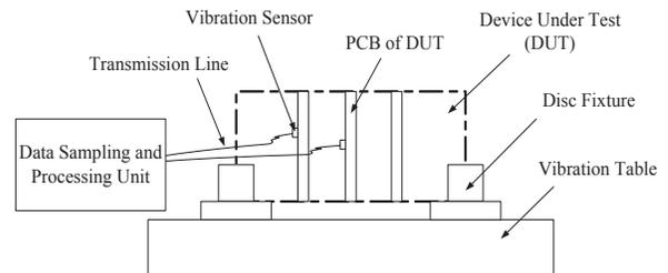
Fig. 2. Equipment installation schematic diagram.
